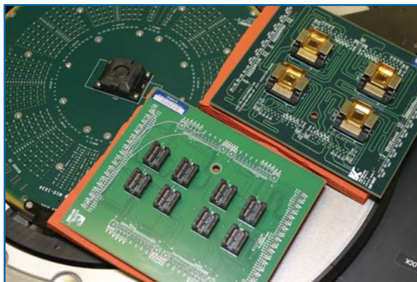
Example: Parallel multi-socket test boards used for greater efficiency
